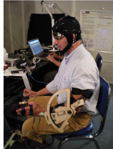
Fig. 2. EEG and fNIR systems are used to monitor brain activity while a subject attempts to distinguish object stiffness using myoelectric control and torque feedback about the elbow.
